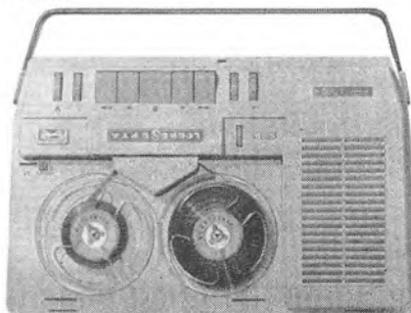
It will accommodate 4½-inch reels, providing a playing time of 60 minutes per track using triple-play tape (1,200 ft.) at the higher speed. Rewind is achieved within two minutes.
