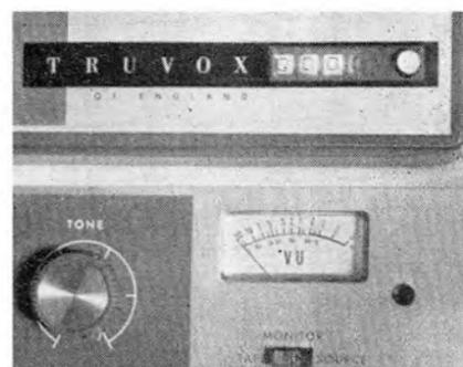
Very accurate VU meters are fitted to the entire Truvox range. The monitor switch (bottom) provides instant flat response comparison between source and tape signal
