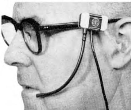
Alternative methods of mounting will enable the unit to be anchored to a helmet or other headgear. A double earpiece assembly is available.
